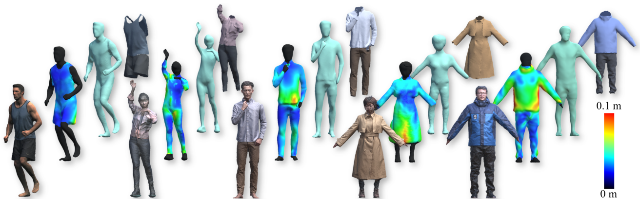
Fig. 8. The gallery of our results. From down to top, the captured meshes, predicted tightness field, recovered body shapes and segmented clothes.
